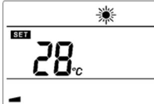
Adjust the desired value with or and wait a few seconds till it is stored automatically.
